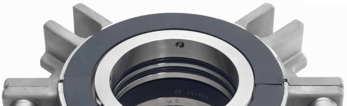
Dynamic test rig with 5.000" (125mm) RDS™ installed
